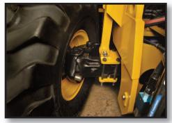
**STEERING CONTROL:** Fully hydraulic power steering with 3 modes (4-wheel, Crab, 2-wheel) provides versatility in the toughest terrains.
