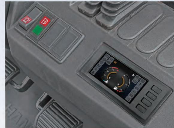
The newly developed LCD instrument display has additional functions and offers more stable performance. Important information including the running status of the entire truck and a check engine light can be displayed. This allows the operator to easily understand the status of the truck for easy maintenance.
