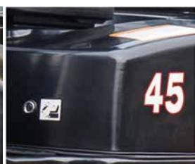
The cover on the Panel can be lifted up simply to check the brake fluid.
