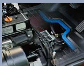
In addition to rubber damper between frames and steering axle, compound engine damper and full floating power train achieve flexible connection between frames and driving system, as a result, traveling vibrations and vibrations from the driving system are significantly reduced.
