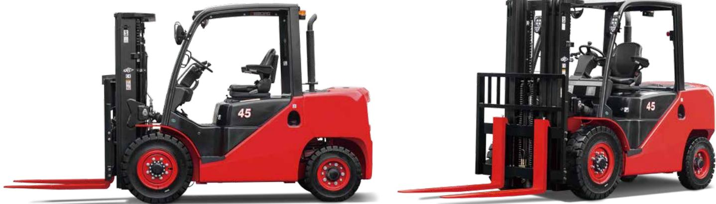
*In developing the XF Series, comfort and ease of operation is carefully considered, for example, to improve vibration levels, compound engine damper and full floating power train are adopted.*
