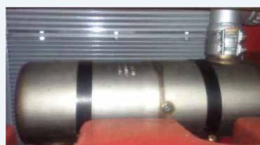
The exhaust treatment DOC ensure the exhaust satisfy with USA T4F , it also with good noise reduction , maintenance is minimal.
