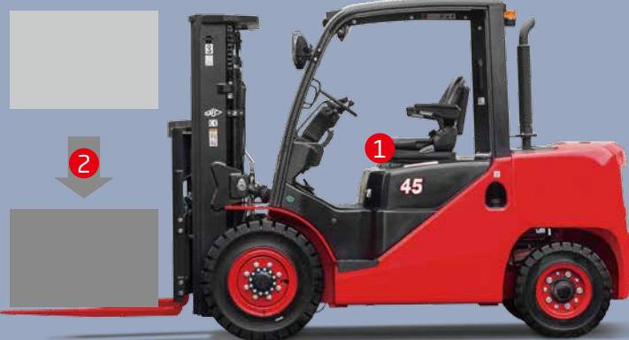
1. The operator presence sensing system incorporates lifting / tilting and traveling locking function. When the operator leaves the seat, the system automatically locks lifting / tilting and disables traveling to ensure safety.
