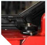
There're four levels shock absorption applied to reduced the vibration from the road to the driver. The damping pad is applied reduce the vibration, Like between the steering axle and the chassis, The engine, torque convertor and the chassis, the overhead guard and the chassis. And the suspension seat is another vibration reduction.
