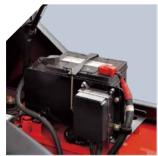
All the controllers, relays, and safety fuses are allocated in the controller box, free to water and dust. The main electronic components are waterproof, which is capable operater in severe environment. And the famous brand air-filter is also applied in the
