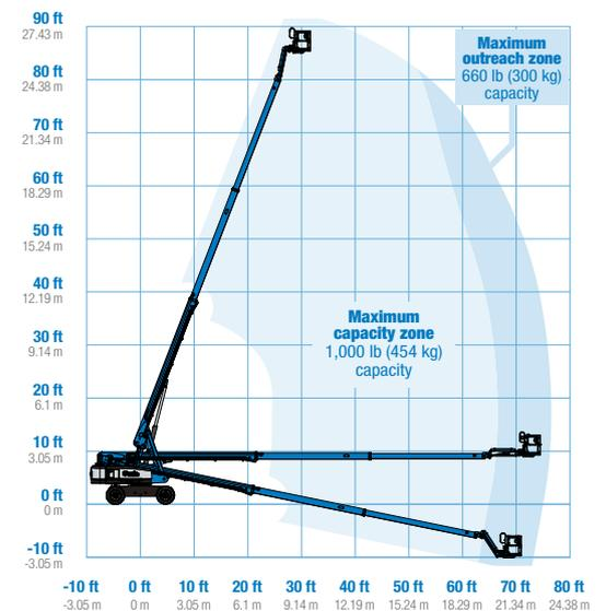
\* The metric equivalent of working height adds 2 m to platform height. U.S. adds 6 ft to platform height.
