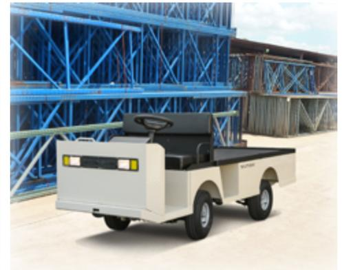
Taylor-Dunn's B-200 is durable, reliable and cost effective for your commercial and industrial material handling needs. Equipped with a 36-volt electric drive train, this vehicle carries loads up to 2,000 pounds at speeds up to 12 miles per hour with a range up to 20 miles.
